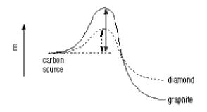
So the trick is to set up the conditions so you form diamond, but not graphite, i.e., you arrange things so the kinetics of the process dominates over the thermodynamics.
