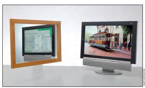
Two-way viewing angle LCD. This new LCD from Sharp Corporation sends the light from the backlight to the right and the left, making it possible to show two different images at the same time. Reflecting the LCD in a mirror shows that one user sees a TV show, while another sees an Internet homepage. One possible application is a car display that shows the driver a map, while the passenger watches a movie on DVD.
