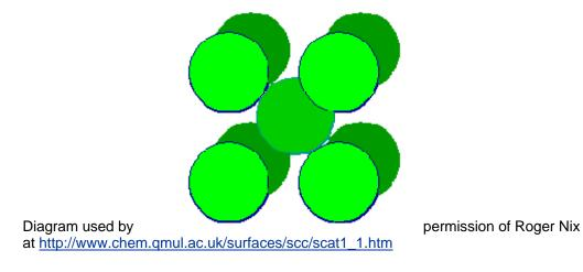
**Face centered cubic (fcc) unit cube** — In a face centered unit cube, 74% of the space is occupied by atoms. The coordination number of each iron atom in this arrangement is 12. A diagram of a face centered cube:
