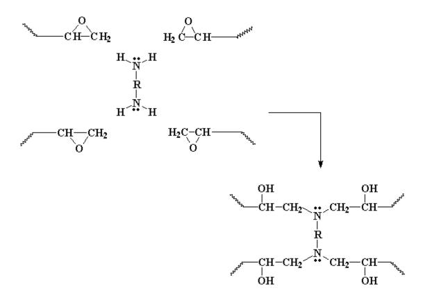
The curing of an epoxy resin to create a material with polar hydroxy groups and amine groups
