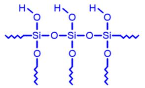
Schematic of silanol groups on the surface of a piece of glass.
