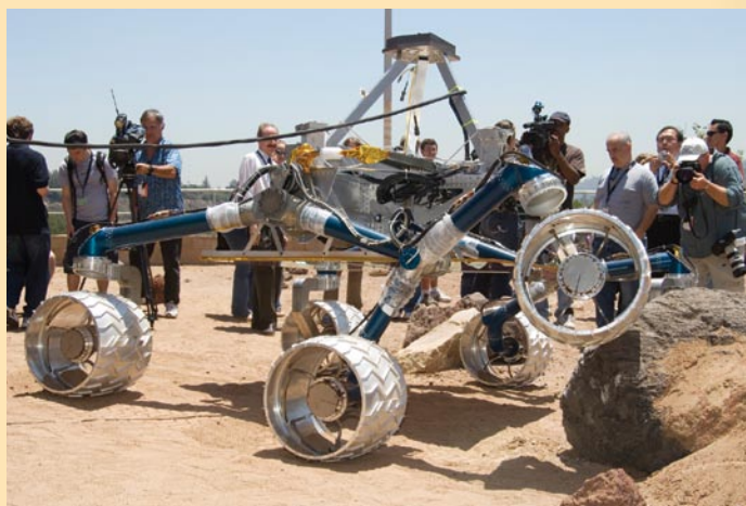
Prototype of the MSL from a test conducted in June 2007 in the “Mars Yard” of the Jet Propulsion Laboratory. The rocks are intended to simulate the shape and size of rocks on Mars that MSL might encounter.
